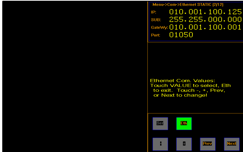
Figure 40 Communication Settings, Ethernet Second Screen
