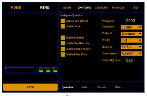
Figure 21 Configure Operation
